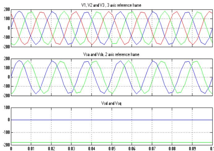
**Fig-13.** The transformation of voltage from three axes to two axes for faulty system
