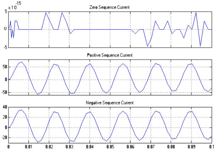
Fig-7. Zero, positive and negative sequence of currents for faulty system
