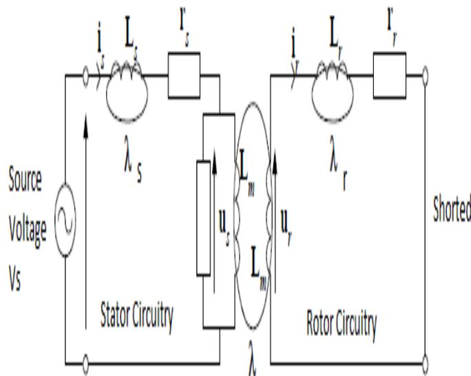
Fig-1. Equivalent electrical circuit of an induction motor
