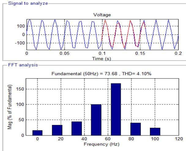
Fig-14. The THD for phase A Voltage for healthy (Unfaulty) system
