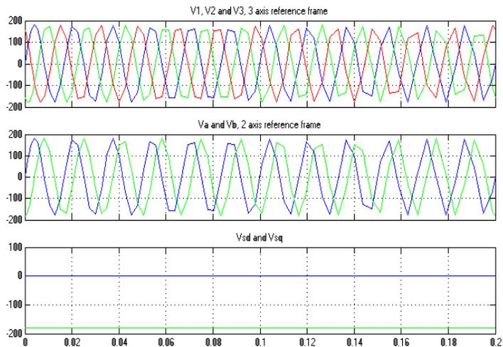
**Fig-12.** The transformation of voltage from three axes to two axes for healthy (Unfaulty) system
