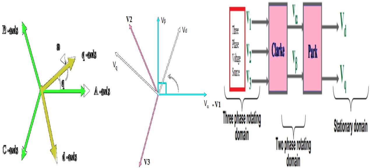
Fig-4. Vector and block diagram of axis transformation using Clarke and Park theories.
