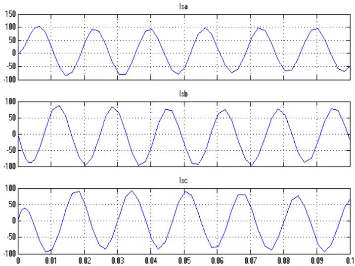
**Fig-11.** The output three phase current of induction motor faulty system
