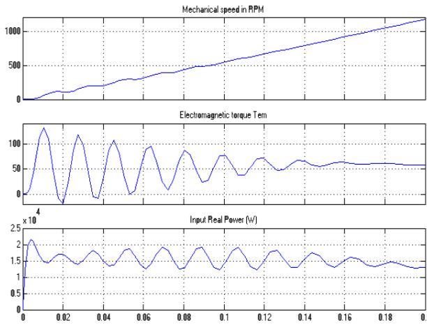
Fig-8. Mechanical speed, electromagnetic torque and input real power for healthy (Unfaulty) system
