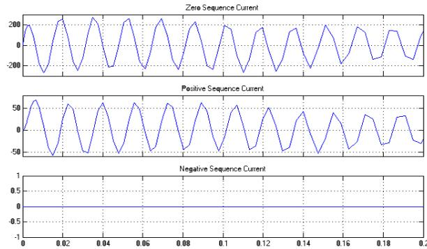
Fig-6. Zero, positive and negative sequence of currents for healthy (Unfaulty) system
