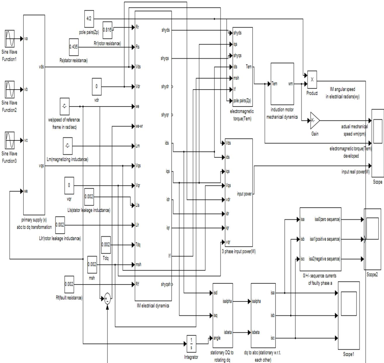
Fig-3. MATLAB Simulink model of Induction Motor.
