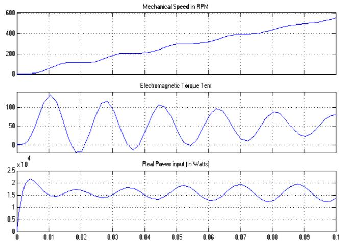
**Fig-9.** Mechanical speed, electromagnetic torque and input real power for faulty system
