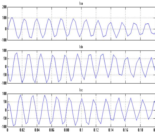
Fig-10. The output three phase current of induction motor for healthy (Unfaulty) system
