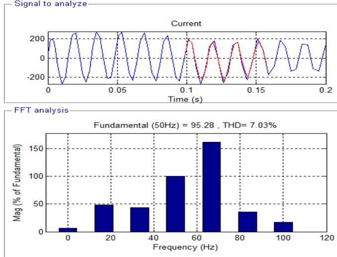
Fig-15. The THD for phase A Current for healthy (Unfaulty) system
