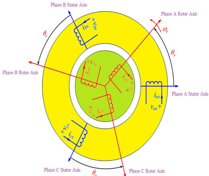
Fig-2. Circuit Model of a Three-Phase IM .
