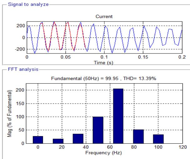
Fig-17. The THD for phase A Current for faulty system
