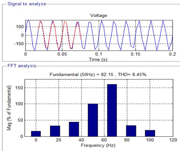
Fig-16. The THD for phase A Voltage for faulty system
