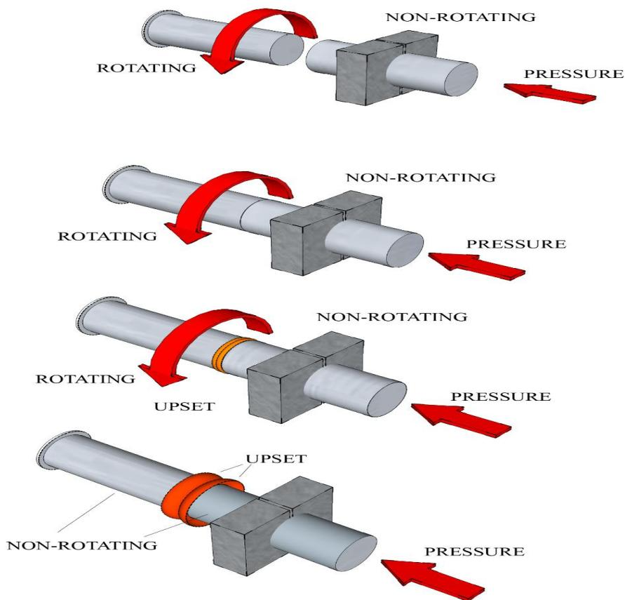
Figure-1. Schematic illustration of friction welding
