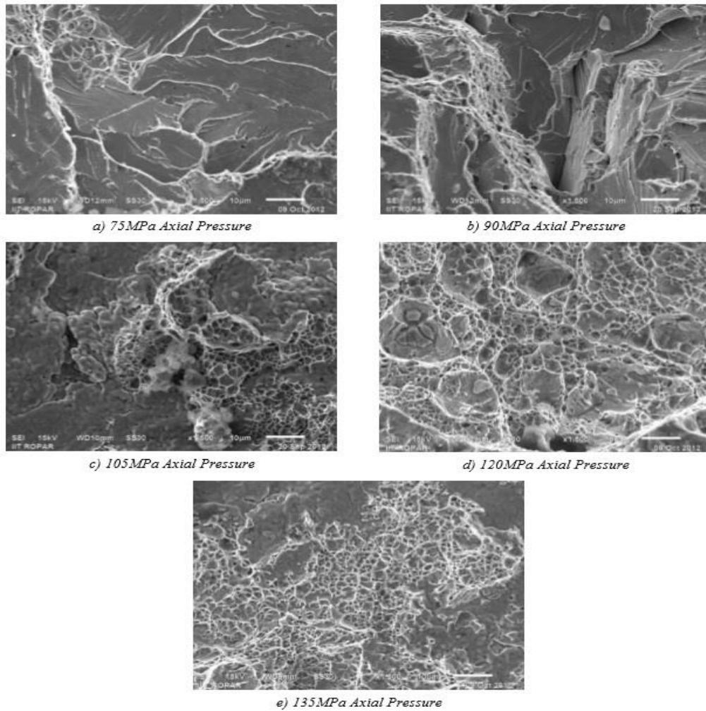
**Fig-2.** SEM micrograph taken at the fractured surfaces during tensile testing of the friction welded specimen welded at 1000 rpm and at different axial pressures
