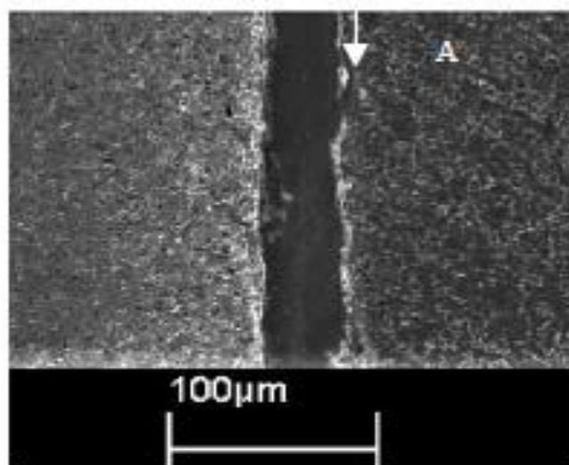
**Fig-3.** SEM micrograph taken from the welding interface of the friction welded specimen welded at 1500 rpm [Ozdemir \[14\]](#)
