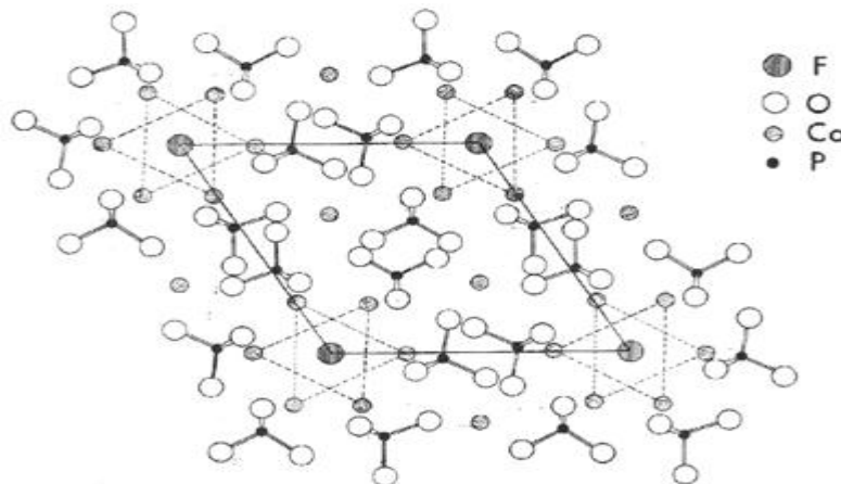
Figure-3. Apatite's structure: atomic arrangement
