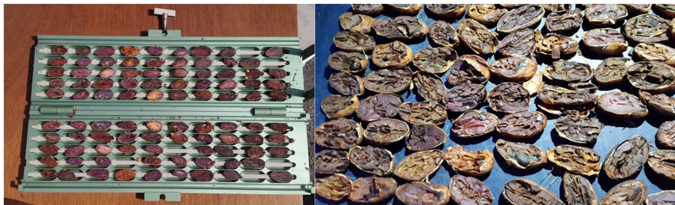
Figure 13. Guillotine for cutting test and guillotined beans showing different defects, and "Light Break" and "Dark Break" beans.
